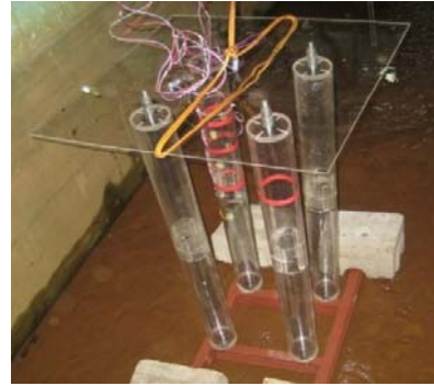
Fig 4(ii) Model with instrumentation - model fitted with accelerometers and strain gauges
