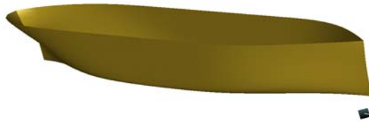
Figure 3: Hull of Series 60 model
